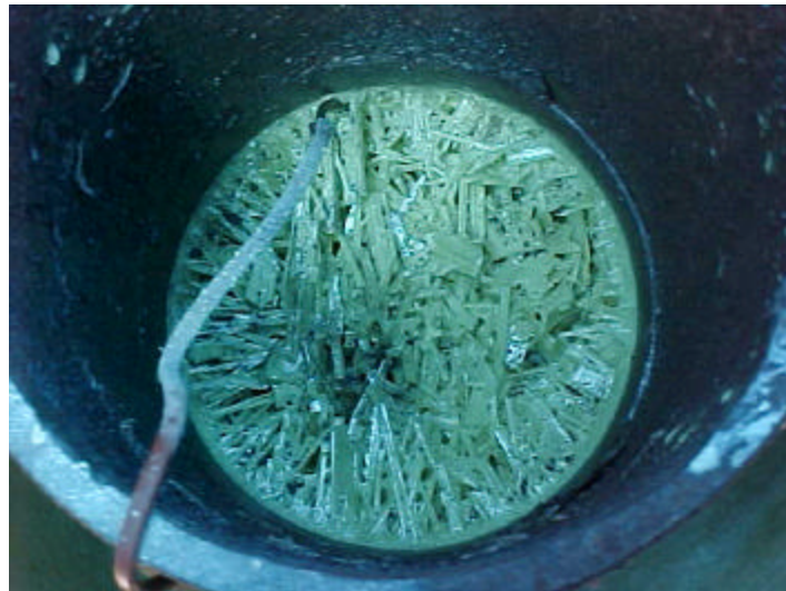
Figure 1 - Sulfur in Its Crystalline State (Top of Fill Pipe)
