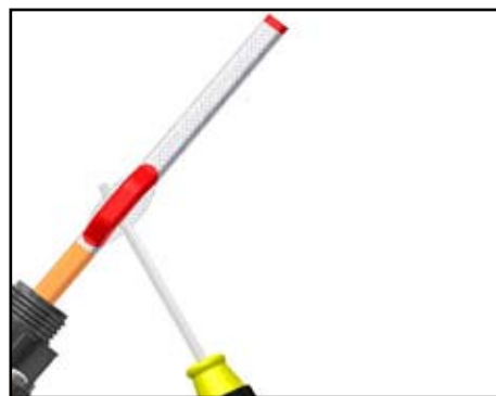
1.6. Separate braid strands at edge of overjacket and pull cable through opening.
