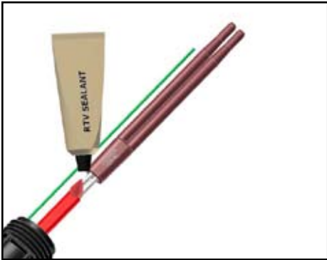
3.10. Apply a liberal amount of RTV sealant to cable.
