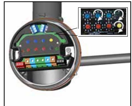
20. Use the rotary switches for setting Control and Limit Temperature, (Celsius or Fahrenheit) and Auto or Manual reset (Control switches on Type "C", Limiter switches on Type "L" and both on Type "CL"). Refer to ECM user manual for further details.
