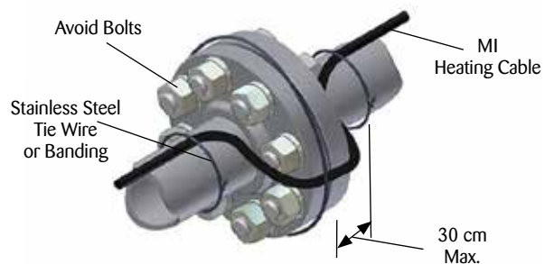
Illustration E: Pipe Flange . . .
