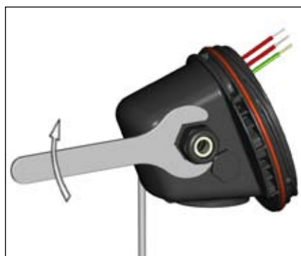
6. Install M25 power gland in M25 threaded entry.
