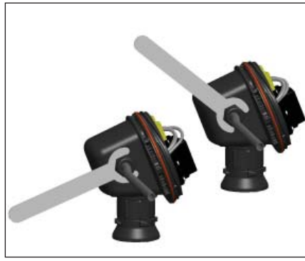
14. Remove M25 dust cap. Install M25 power gland (order separately) and M25 blind plug. For in-line splice, T-splice, or end termination, install additional M25 blind plug (order M25-B-EXE separately) instead of M25 power gland.
