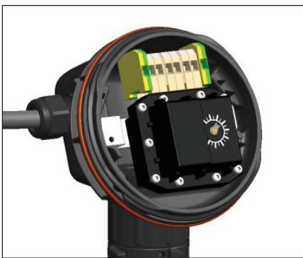
16. Install thermostat and complete system wiring. Terminal set screws shall be tightened to a torque value of 1.4 Nm (12.4 lb-in). See page 4 for wiring details. Set thermostat at desired setpoint.
