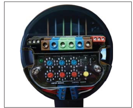
11. Install electronic control module and complete system wiring. Terminal set screws shall be tightened to a torque value of 1,4 Nm (12,4 lb-in). See wiring details. Set modules electronic control and/or control limiter at desired setpoints.
