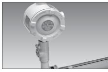
**D1-ECK kit** is required for power connection and heating cable termination in Class I, Division 1 hazardous (classified) areas. D1-ECK-2 kits for in-line splices and D1-ECT kits for T-splices are also available.
