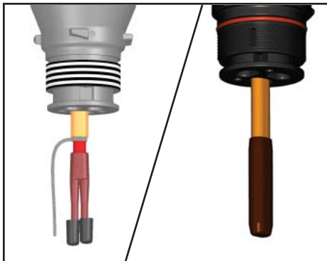
12. Completed heat tracing termination. PETK kit for Power/End Terminations
