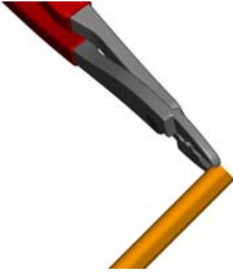
A1. Cut off end of cable.
