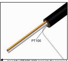
Insert the PT100 (150 mm) into the prepared hole, between the tube(s) and the thermal insulation.
