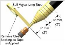
11. While removing the clear backing from tape, wrap end of tubing bundle with selfvulcanizing tape. Start a minimum of 51mm (2") above the cut on the outer jacket and continue a minimum of 51mm (2") along the bare tubing. Overlap the tape at least 50%. It is recommended that the heater end terminations be sealed and placed inside the insulation or at the connection, to assure no moisture enters the bundle insulation.
