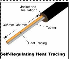
Trim heat tracing to within 305mm - 381mm of the end of the insulation. If self-regulating heat trace proceed to step 3. For Zone-type heat trace continue with identification of bus connection on step 2a.
