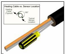
Prepare tubing bundle for PT100 sensor by inserting a phillips screwdriver a minimum depth of 150 mm (6") between the process tube(s) and insulation at a point opposite the heating cable. The sensor should be placed 180° around the circumference from the heating cable. Make sure that the entire length of the sensor is in intimate contact with the tube surface. Prevent kinking.
