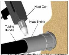
ris recommended that the tubing, heat trace (where included) and other connections be made before completing this step. Heat until heat shrink seal is conformed and sealed to the tube bundle outer jacket.
