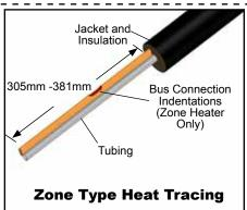
2a. Strip back bundle insulation 38mm to 76mm beyond bus connection heat tracing. If bus connection indentation is a less than 305mm -381mm from end of! the heat tracing, proceed stripping the bundle insulation to the next indentation.
