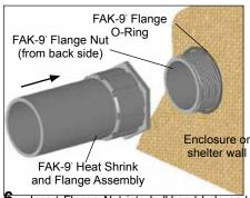
Insert Flange Nut into bulkhead hole and engage Flange Assembly as shown. Tighten firmly by hand. If further tightening is desired, use suitable spanner wrench ensuring not to over-tighten as Flange Nut can be broken.
