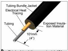
Strip back insulation approximately 101mm (4") from tubing bundle end .
