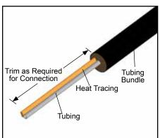
Remove outer jacket and insulation from tubing bundle to expose the electric heat trace and tubing. Ensure sufficient heat trace is available for electrical connection. See instructions included with heat trace PETK kit.
