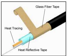
Wrap tubes and heat tracing with pass of heat reflective tape (25% overlap). Then wrap with 3 passes of glass fiber tape (50% overlap), or until fiber tape is equal to original bundle insulation thickness. See steps 9, 10, and 11 for bundle end seal using FAK-7.
