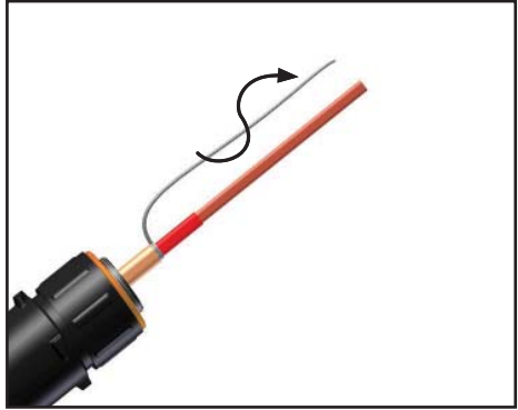
1c. Twist braid into a pigtail. Trim ends of braid.
