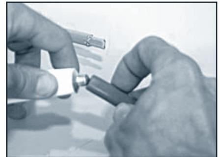
**Step 15:** Fill the smaller end cap with RTV.
