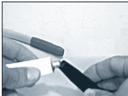
**Step 17:** Put a small amount of RTV into the opening of the larger over-cap.
