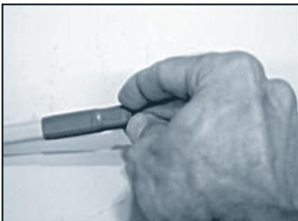
**Step 16:** Slide the end cap on the end of the cable until fully seated.
