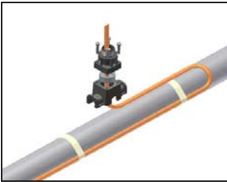
1.1a. For one, two or three cables. Insert cable into expediter, grommet, and NPT threaded cap.
