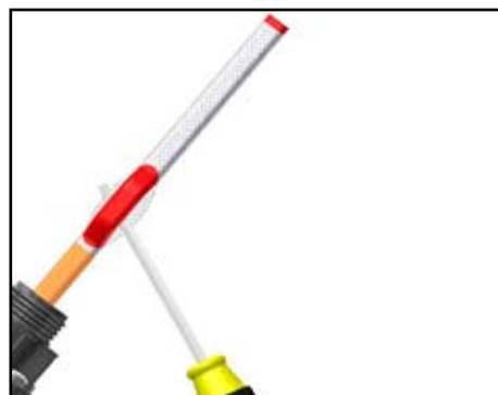
1.6. Separate braid strands at edge of overjacket and pull cable through opening.
