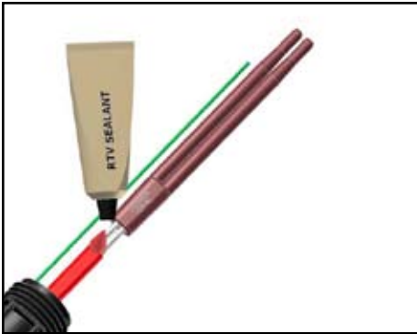
3.10. Apply a liberal amount of RTV sealant to cable.
