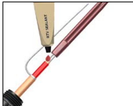
1.12. Apply a liberal amount of RTV sealant to cable.
