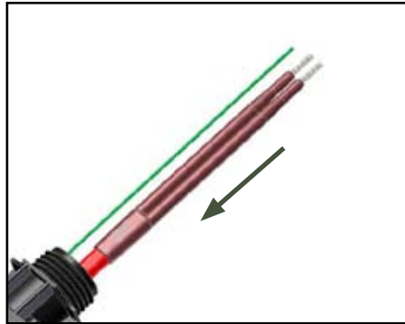
3.11. Slide boot onto the end of the cable.
