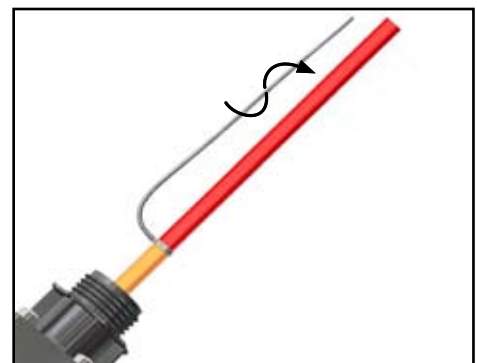
1.7. Twist braid into a pigtail. Trim ends of braid.
