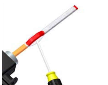
1.5. Separate braid strands at edge of overjacket and pull cable through opening.
