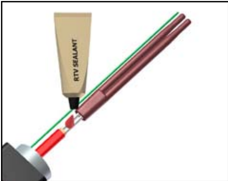
3.9. Apply a liberal amount of RTV sealant to cable.
