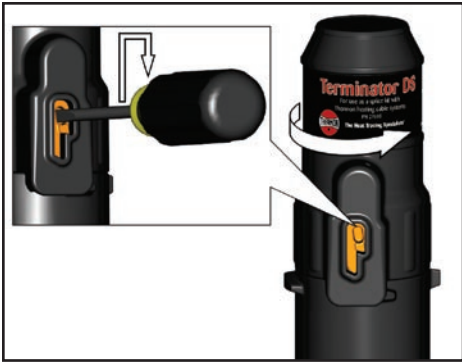
12. To remove cap, lift latch mechanism and unscrew cap.
