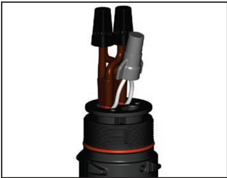
9. For splice connections: Connect bus wires using small wire nuts (for BSX, HTSX, KSX and TSX) or medium wire nuts (for RSX, VSX, HPT and FP). Connect braid wires using large wire nut. See wiring details for splice connections.
