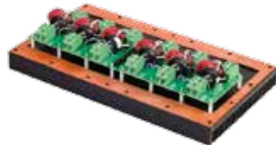
Power Output Module (polycarbonate cover not shown)
