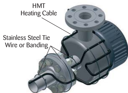
Heating Cable Serpentine on Pump
