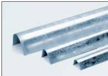
**TFK-4** galvanized steel channel 1.18" x .84" (30 mm x 21 mm) covers SnapTrace heat transfer compound applied to 3/8" or 1/2" O.D. tube tracers.
