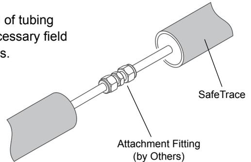
3. Wrap glass fiber tape until level with SafeTrace insulation. Wrap heat reflective tape over fiber tape (25% overlap).
