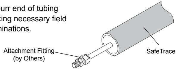
3. Liberally apply RTV sealant to end of SafeTrace insulation.
