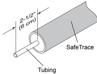
2. Deburr end of tubing making necessary field terminations.
