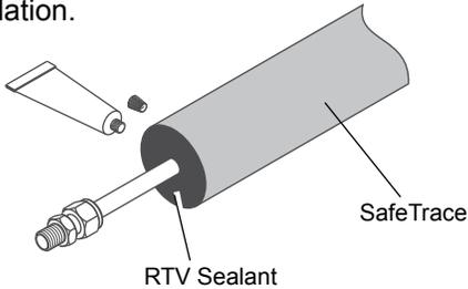
4. Wrap end of SafeTrace with silicone tape. Overlap the tape 50%, beginning 2½" (6 cm) over SafeTrace insulation extending to the attachment fitting.
