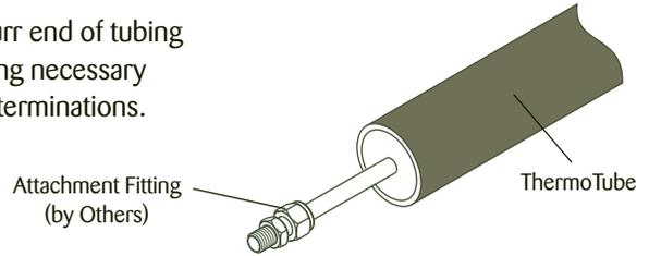
3. Liberally apply RTV sealant to end of ThermoTube insulation.
