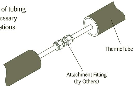
3. Wrap glass fiber tape until level with ThermoTube insulation. Wrap heat reflective tape over fiber tape (25% overlap).
