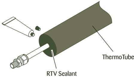
4. Wrap end of ThermoTube with silicone tape. Overlap the tape 50%, beginning 2½" (6 cm) over ThermoTube insulation extending to the attachment fitting.
