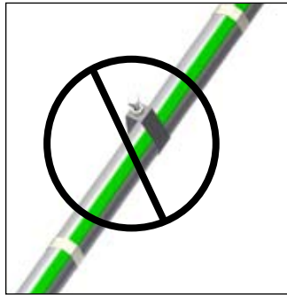
Do Not Install Cable Like This:
