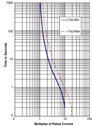
**Fig. 5: Typical North American Breaker Trip Curve**
