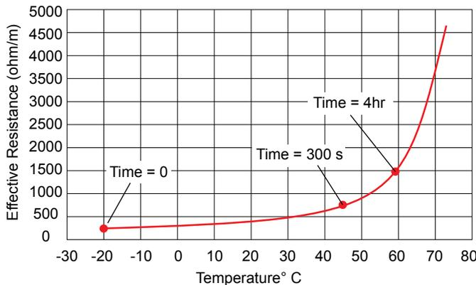
**Fig.4: Effective Resistance vs. Tracer Temperature & Time**
