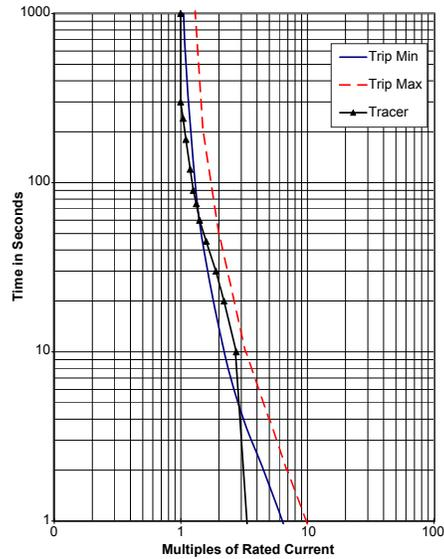
**Fig. 8a: Typical North American Breaker Trip Curve**
