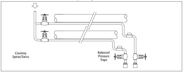
Figure 10 Isolated Steam Tracer for Temperature Control
